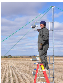
Rick Engel in Hill County, MT standing in front of ammonia sampling device
