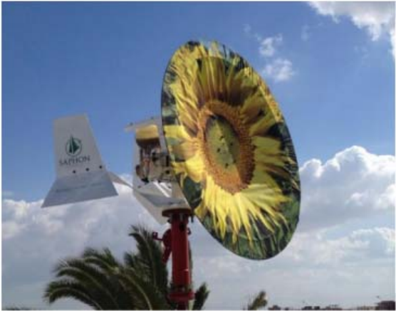
Figure 7a: Bladeless wind turbine design
