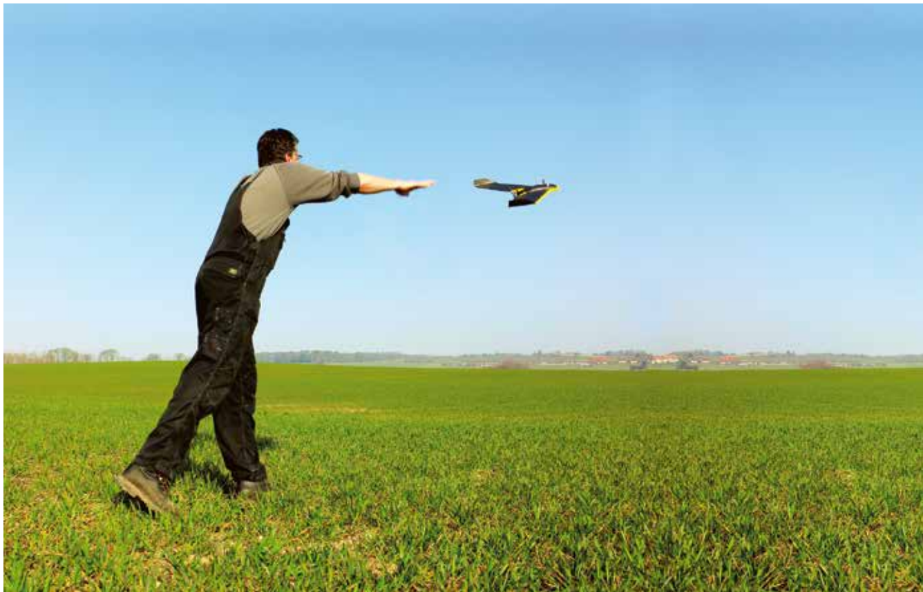
An operator launches the senseFly eBee, a professional mapping drone. Use this fully autonomous drone to capture high-resolution aerial photos that you can transform into accurate 2D orthomosaics & 3D models.. Photo courtesy of senseFly.
