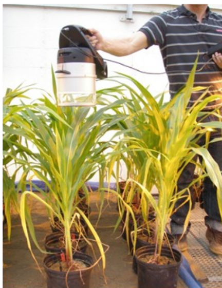
Figure 1. Operator holding the Multiplex sensor for corn fluorescence readings.
