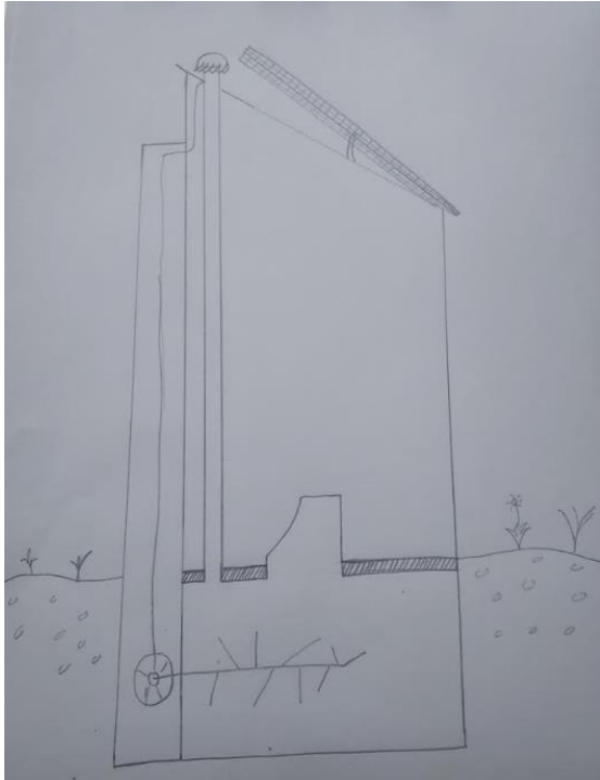
Figure 4. A sketch of the proposed MSU “M” vent toilet design. Sketch by author: Esther Maina.
