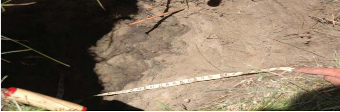
Figure 3.4: Soil Profile Three, with silt-sized alluvial deposits overlying a buried A- horizon
