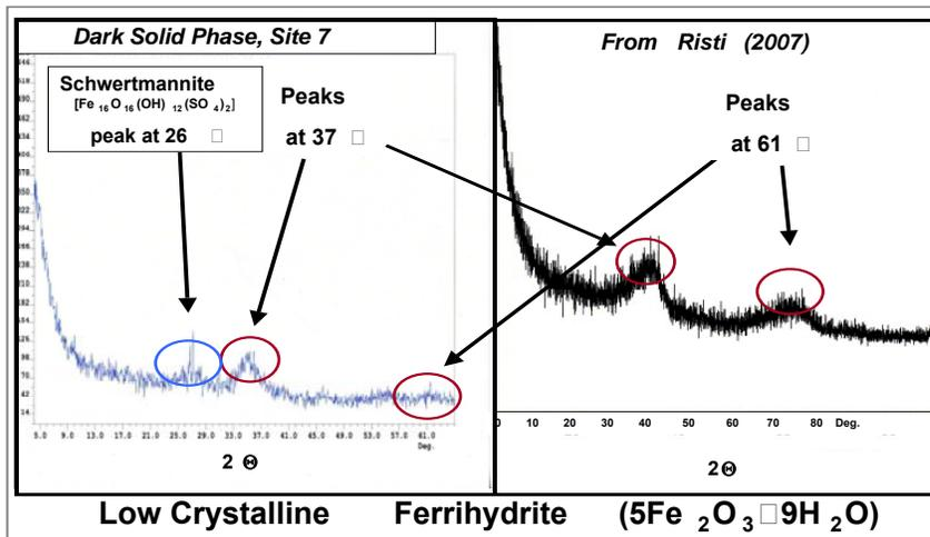
Figure 14. XRD output indicating the presence of amorphous ferrihydrite and Schwertmannite in the Alta Mine solid phase samples. XRD data in right panel is of a pure ferrihydrite and is from Risti (2007).
