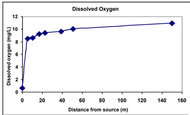
**Figure 10.** Dissolved oxygen content as a function of distance from adit.
