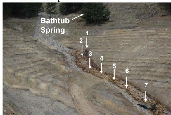
**Figure 9.** Aqueous and solid phase chemistry sampling sites.
