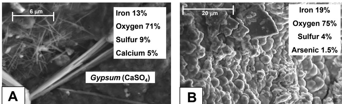
Figure 13. SEM-EDAX analysis of Fe solid phase samples from the Alta Mine outflow channel. (A) highly crystalline sample exhibiting elemental content consistent with gypsum; (B) amorphous Fe-oxy-hydroxides containing some sulfur and arsenic.
