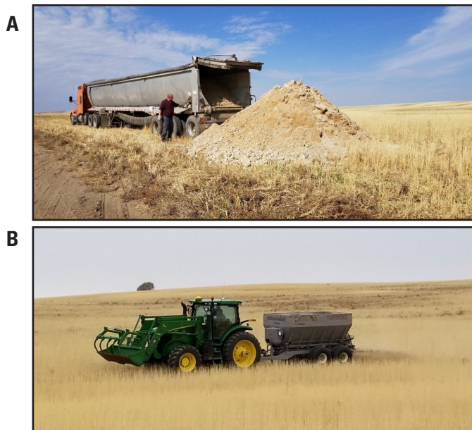
Figure 1. Beet lime was trucked to field locations (A), and then distributed with a Stoltzfus wet-lime applicator (B).
